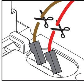
Remove the red (positive) and brown (negative) cables with fastons from the diode bridge.
