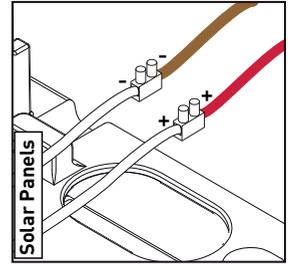
Connect the 24V solar panel cables = (not supplied), the negative to the brown wire (-) and the positive to the red wire (+).
