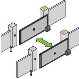
With these settings, command 1-3 starts an opening operation of the automation that it is connected to which will close after the time set with **BA > TC**. Once the delay time set with **AP > TO** has elapsed, the other automation will open and will close after the time set with **BA > TC**.
