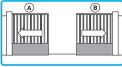
With the parallel connection, the opening, closing, reopening when an obstacle is encountered during closing and flashing of flashing lights are synchronised. The obstacle during opening and safety devices (safety edges) must be installed each one on its own door and act independently of each other.
