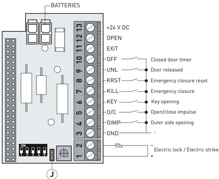
**i** Fix the label to the terminal board, taking care to apply it in the correct direction (see the figure above).
