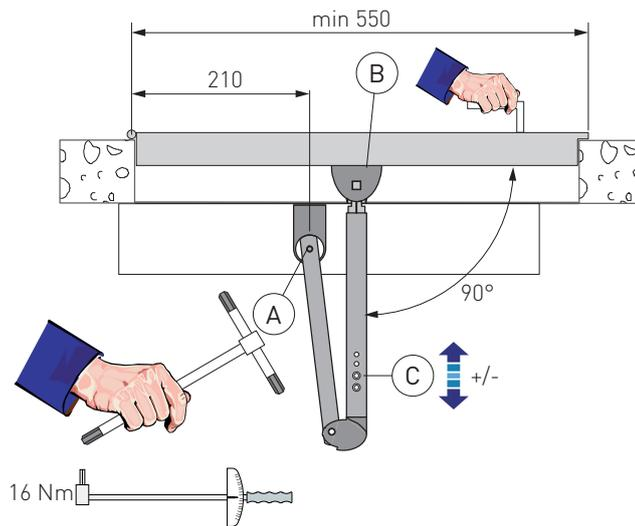
**NB:** open the door slightly and tighten the screw of the arm support seat [A] at 16 Nm (as shown in the figure).
