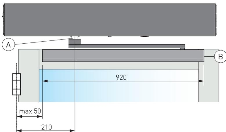
**NB:** open the door slightly and tighten the screw of the arm support seat [A] at 16 Nm (as shown in the figure).
