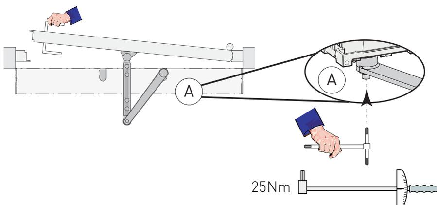
**NB:** open the door slightly and tighten the screw of the arm support seat [A] at 25 Nm (as shown in the figure).
