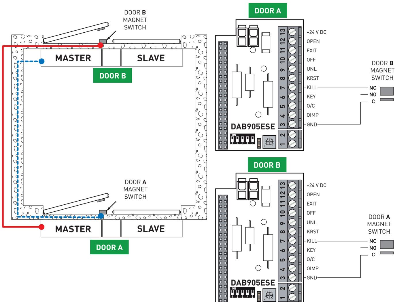
In applications for interlocked doors, a micro switch must be installed on the MASTER A automation in order to disable opening of the MASTER B automation and vice versa.
