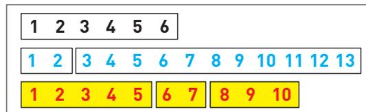
**i** Remove the jumpers if a safety sensor is connected to terminals 1-2 and 1-3.
